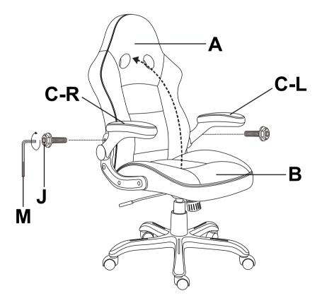
Note: Push the Back Cushion (A) to the upright position. Assemble 2x Screws (J) into the top holes of Back Cushion (A).
