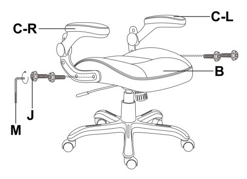
Note: Attach Armrests (C) to the assembled Seat Cushion (B) using 4x Screws (J) with Allen Wrench (M). Do not tighten Screws fully until you have completed assembly.
