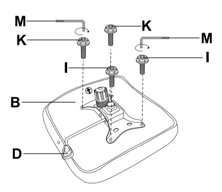
Note: Align the Seat Plate (D) so the FRONT of the Seat Plate matches the FRONT label on the bottom of the Seat Cushion (B). Tighten the screws.
