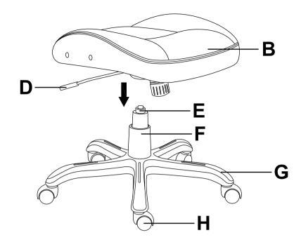
Note: Place assembled seat on the Gas Lift (E). Push down firmly until connection is secure.
