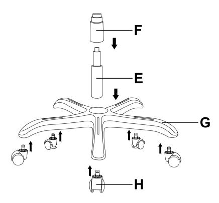
Note: Turn the Star Base (G) upside down. Press the Casters (H) into holes at the end of each leg. Turn the Star Base (G) upright and insert Gas Lift (E) into the center hole of Star Base (G). Gas Lift Cover (F) should be in place over Gas Lift (E).
