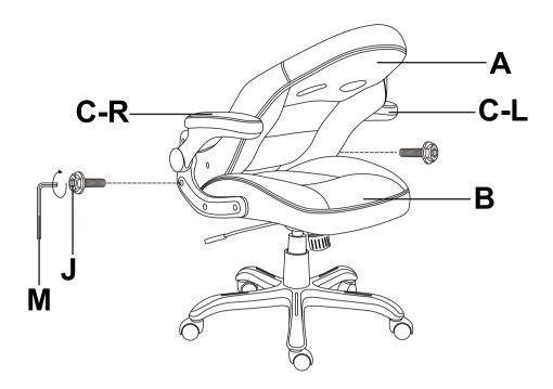
Note: Attach Back Cushion (A) to Armrests (C) by securing 2x Screws (J) to the lower holes of the Back Cushion (A) as shown. Do not tighten Screws fully until Step 7.
