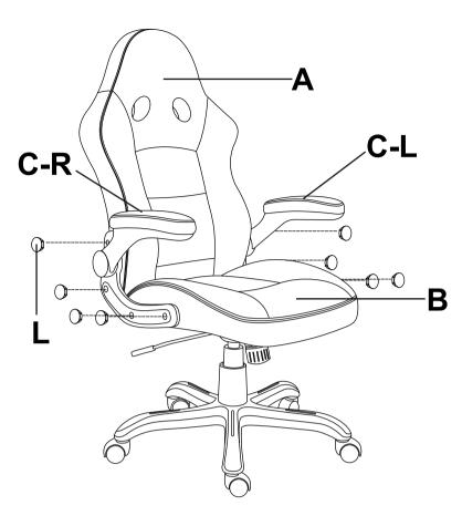
Note: Fully tighten all Screws (J) with Allen Wrench (M). Press the Plastic Caps (L) into the Armrest holes to cover the screws.
